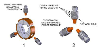
Figure 32 Some configuration of clutch spring stack. Each 'spring' stack contains multiple springs (Belleville washers) - arranged into three, four, or five 'flying saucers', or turned away against the flat washer(s). Shown is the  $4\frac{1}{2}$  stack..
