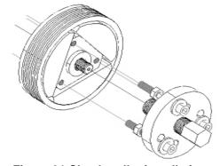
Figure 31 Clutch puller installation
