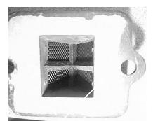
Figure 44 The presence of light may indicate that the reeds may need to be replaced, or possibly turned over.
