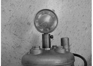
**Figure 36,** Using a dial indicator to measure piston height for setting ignition timing.
