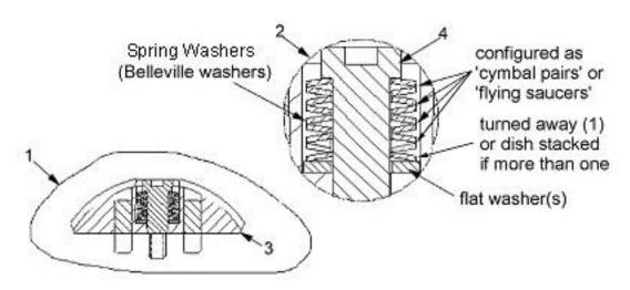
**Figure 32 Some configuration of clutch spring stack**. Each 'spring' stack contains multiple springs (Belleville washers) - arranged into three, four, or five 'flying saucers', or turned away against the flat washer(s). Shown is the 4 ½ stack.
