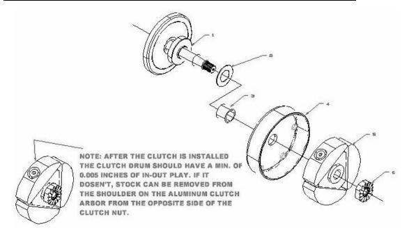
Figure 33, Clutch Assembly Drawing
