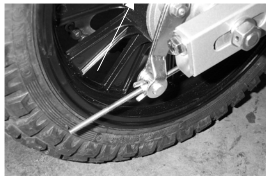
Figure 7 , adjust lever 'free play'
