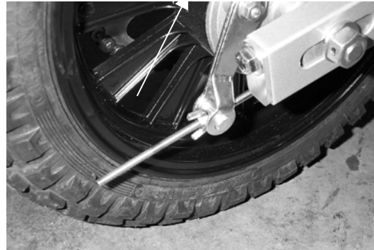
Figure 7, adjust lever 'free play'
