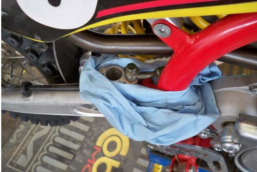
Step 7: Place a protective wrapping around the master cylinder and frame.
