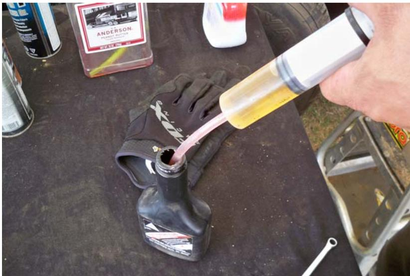
Step 6: Fill the syringe with brake fluid and make sure the feed tube is free of air.
