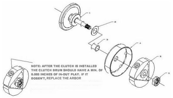
Figure 33, Clutch Assembly Drawing
