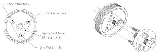
Figure 30 Figure 31 Clutch puller installation Tools recommended for clutch service:
