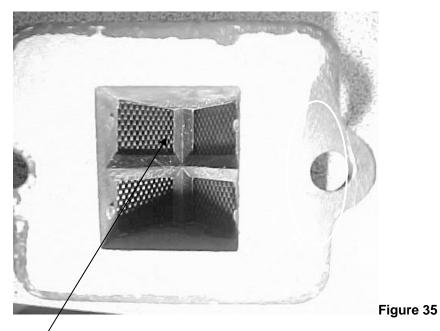
The presence of light indicates that the reeds should be replaced, or possibly turned over.
