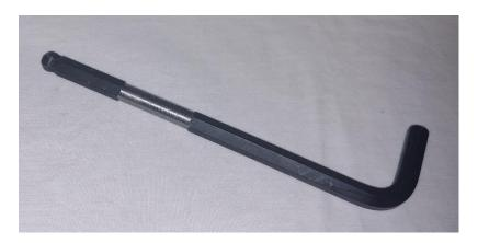
For draining the oil, use the short end to break it lose. Then use the ball driver end stuck through the hole in the brake pedal to quickly easily turn out the drain plug.
