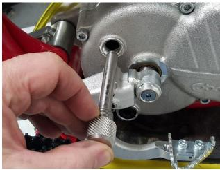
To properly measure the minimum torque at which the CFD (Cobra Frictional Drive) slips
