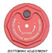
The Smart Leg cap is labeled "Speed Sensitive Bottoming Control", and this adjuster provides a range of control over how progressive the fork feels. Turning the screw clockwise increases the fork's resistance to bottoming, while turning the screw counter-clockwise decreases it. On the track, this effect will be felt on sections where the fork is forced to move very quickly such as on harsh landings or when traversing sharp edged bumps.
