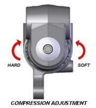
At the base of the conventional leg is another adjustment screw that controls the amount of compression damping. Turning this screw clockwise increases damping and turning it counter-clockwise will decrease it. This is illustrated by the "HARD" and "SOFT" in the figure at the right.
