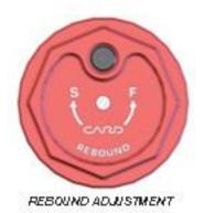
The speed at which the fork rebounds can be adjusted at the top of the conventional leg. Turning the adjustment screw clockwise slows the rate at which the fork extends after being compressed, and likewise,
