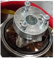
**NOTE**: It may be helpful to use a screwdriver or similar device in the side hole of the puller to stop rotation
