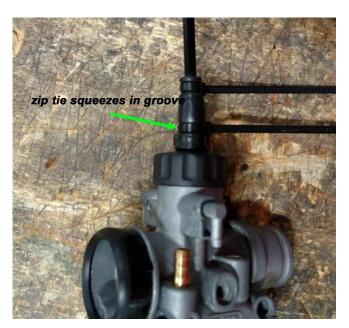
NOTE: For the strongest grip, the bottom (left in the pictures) zip tie should be squeezing on the groove between the hex adjuster and the top, NOT the groove in the carb top.
