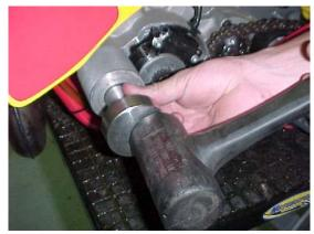
11. Continue driving the assembly with the punch until the head is flush.
