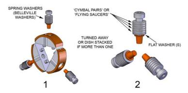
**Figure 38 Some configuration of clutch spring stack**. Each 'spring' stack contains multiple springs (Belleville washers) - arranged into three, four, or five 'flying saucers', or turned away against the flat washer(s). Shown is the 4 ½ stack..
