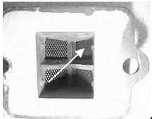
Figure 46 The presence of light indicates that the reeds should be replaced, or possibly turned over.
