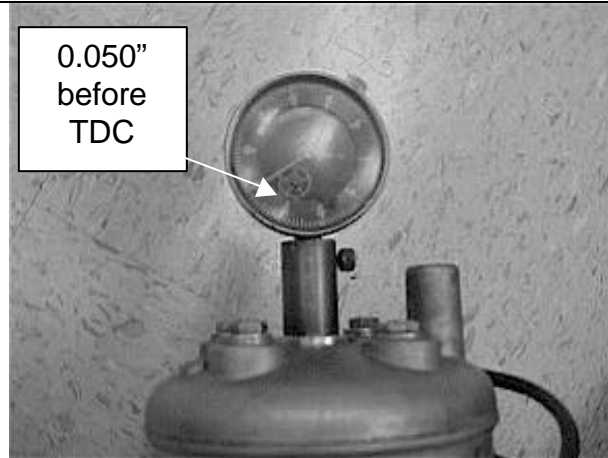
Figure 21 , Using a dial indicator to measure piston height for setting ignition timing.
