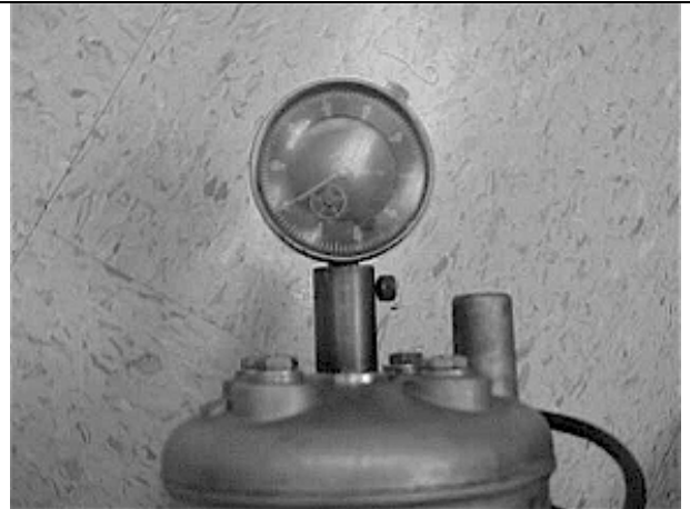
Figure 38 , Using a dial indicator to measure piston height for setting ignition timing.
