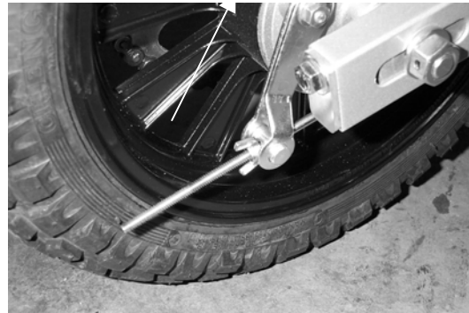
Figure 7 , adjust lever 'free play'
