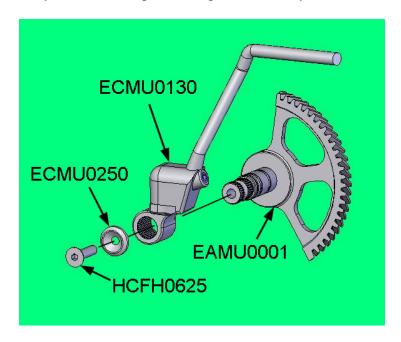
If the threads strip out of the ECDC0046 swivel, a longer bolt with a nut may be an option, or likewise a heli-coil, may be a cost effective alternative to purchasing a new kick lever and gear.
