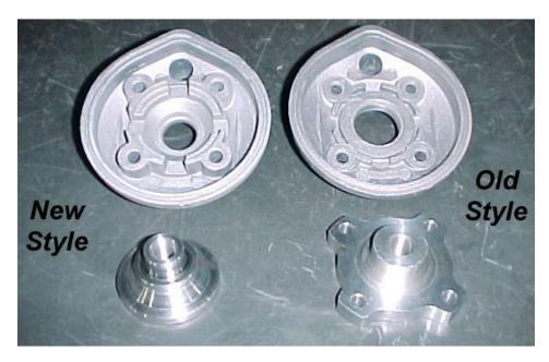
The two configurations require different top-end o-ring sets. The table on the following page will help sort and organize gasket kits for these and earlier models.
