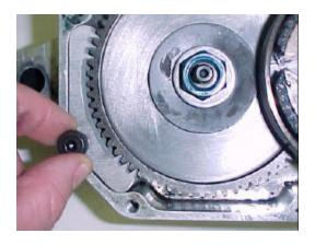
Using a beam style torque wrench, turn the torque wrench counter clockwise and observe the torque measurement when the shaft slips relative to the gear. Using a preset value torque wrench, adjust the setting **55 ft-lb (75 Nm)** and observe whether the wrench clicks first or the shaft slips. If the shaft slips first, the slip torque is below 50 ft-lb and the CFD needs servicing. If the wrench clicks first, the CFD is of acceptable value.
