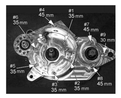
Proper torque is 80 in-lb (9 Nm).
