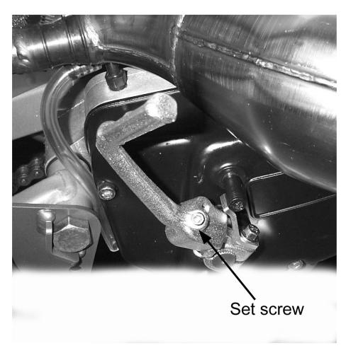
It is advisable to install some thread locking agent to the threads of the set screw when it is adjusted to the desired setting (set screw positioning in and out determines the ease with which the kick lever can be rotate into position).
