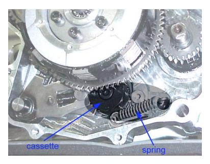
All units produced of Revision 1.4 and higher will have this upgraded hardware direct from Cobra. Customers with units produced prior to Rev 1.4 may call into Cobra and arrange an upgrade of cassette and spring. This will require the customer to receive a proper Return Authorization number (RA#) prior to sending in their cassette. It is suggested to retain the lighter spring as some riders prefer the light feel of the original spring.
