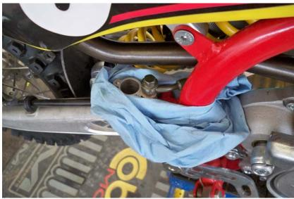
Step 7: Place a protective wrapping around the master cylinder and frame. **Caution**: Silicone brake fluid can damage paint and other finishes, so be careful.
