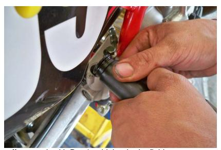
Step 4: Top off reservoir with Dot 4 or higher brake fluid.
