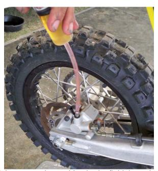
Step 8: Back bleed the system by pushing brake fluid through the caliper and into the master cylinder. Allow fluid to spill over the top of the master cylinder until no more air bubbles emerge.
