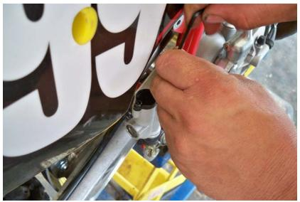
Step 2: Remove the reservoir cap with a 3mm hex key.
