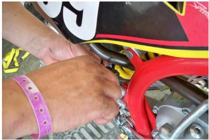
Step 9: Tighten the bleed screw, top off fluid, and replace the master cylinder cover. Depress the brake lever by hand a few times...it should immediately feel better. Repeat the process if you feel air is still trapped.
