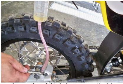
Step 5: Use a syringe or other suitable device to vacuum bleed the system. Make sure that enough fluid stays in the reservoir so as to not pull any more air into the system.
