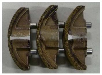
These shoes require a slightly different spring stack as compared to the other shoes. They tend to work better with 0.010" (0.25mm) more shim height. If you have received washer stacks with just a single 0.010" (0.25mm) shim, we suggest that you replace the .010" (0.25mm) shim with a .020" (0.50) shim, or add a 0.010" (0.25mm) shim to the original one.
