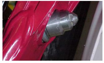
To avoid solenoid rotation, it may be necessary to squeeze the solenoid body with a tool.
