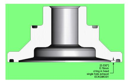
Please take care when building a 60cc mod engine to know what head insert is required for your application. Picking the wrong insert can result in poor performance and/or an expensive engine failure.
