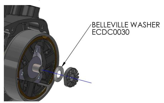
As before, torque the clutch nut to 45 ft-lb with red high strength thread lock agent (Loctite 263).
