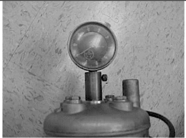
Figure 27 , Using a dial indicator to measure piston height for setting ignition timing.
