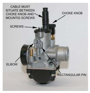
**Figure 34** Proper carburetor top installation and location of rectangular slide indexing pin and vent elbows.
