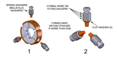
**Figure 32 Some configuration of clutch spring stack**. Each 'spring' stack contains multiple springs (Belleville washers) - arranged into three, four, or five 'flying saucers', or turned away against the flat washer(s). Shown is the 4 ½ stack..
