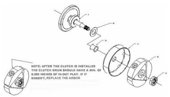
Figure 33, Clutch Assembly Drawing
