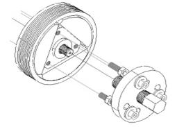
Figure 31 Clutch puller installation
