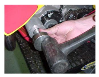
11. Continue driving the assembly with the punch until the head is flush.
