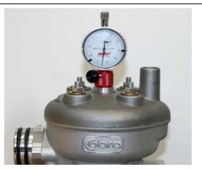
**Figure 27,** Using a dial indicator to measure piston height for setting ignition timing.
