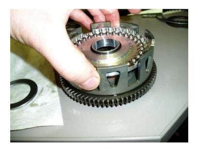
c. Place the thrust plate against the balls on top of the pressure plate. Make sure the 4 outer tabs do not rest in the same basket slots as the 4 outer tabs of the Pressure Plate. The machined side of the thrust plate must face up/away from the balls.
