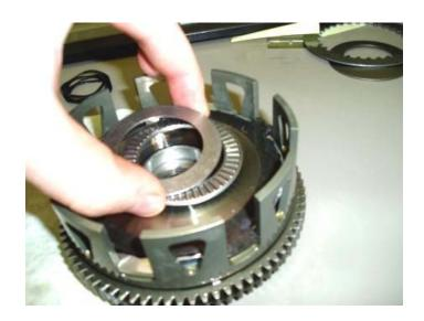
e. Install the clutch pack starting with a friction (fiber) plate and ending with a steel drive plate. Use 5 fibers, 2 x 1.2mm (0.047") steels, 2 x 1.4mm (0.055") steels and 1 x modified steel plate.
