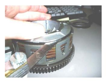
h. Once the proper gap is achieved, install the **new 35MM long clutch center bolt** with spring washer and torque to 40 ft-lb (54 Nm).
