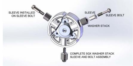
**Figure 32 Some configuration of clutch spring stack**. Each 'spring' stack contains multiple springs (Belleville washers) - arranged into three, four, or five 'flying saucers', or turned away against the flat washer(s). Shown is the 5 ½ stack.
