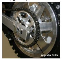
3. Sit on the bike and verify that the chain has a minimum of 12mm (1/2") free movement when the chain is at its tightest point.
