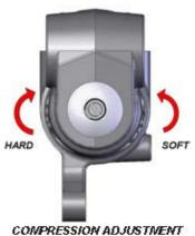
At the base of the conventional leg is another adjustment screw that controls the amount of compression damping. Turning this screw clockwise increases damping and turning it counter-clockwise will decrease it. This is illustrated by the "HARD" and "SOFT" in the figure at the right.
