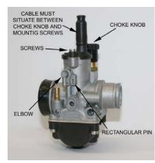
**Figure 45** Proper carburetor top installation And location of rectangular slide indexing pin and
