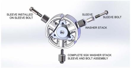
**Figure 32 Some configuration of clutch spring stack**. Each 'spring' stack contains multiple springs (Belleville washers) - arranged into three, four, or five 'flying saucers', or turned away against the flat washer(s). Shown is the 5 ½ stack..
