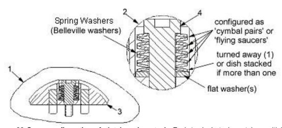
**Figure 32 Some configuration of clutch spring stack**. Each 'spring' stack contains multiple springs (Belleville washers) - arranged into three, four, or five 'flying saucers', or turned away against the flat washer(s). Shown is the 4 ½ stack..
