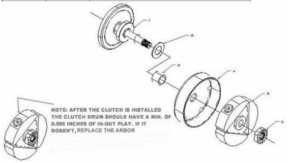
Figure 33, Clutch Assembly Drawing
