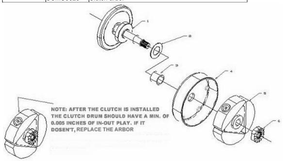
Figure 33, Clutch Assembly Drawing
