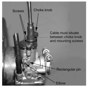
Figure 34 Proper carburetor top installation and
