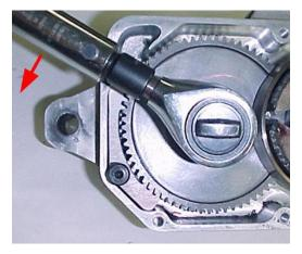
Using a beam style torque wrench, turn the torque wrench counter clockwise and observe the torque measurement when the shaft slips relative to the gear. Using a preset value torque wrench, adjust the setting **55 ft-lb (75 Nm)** and observe whether the wrench clicks first or the shaft slips. If the shaft slips first, the slip torque is below 55 ft-lb and the CFD needs servicing. If the wrench clicks first, the CFD is of acceptable value.
