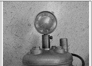
**Figure 27**, Using a dial indicator to measure piston height for setting ignition timing.
