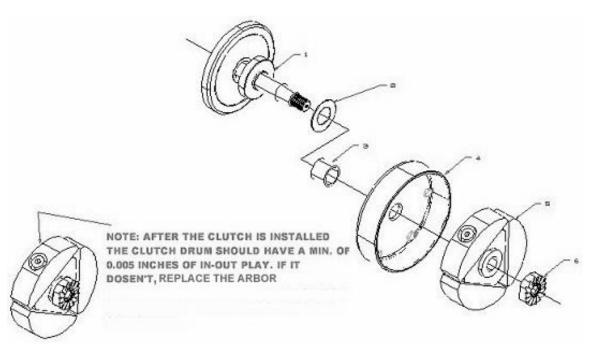
Figure 33, Clutch Assembly Drawing
