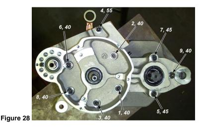
8. Insert the case screws with the proper lengths at locations shown.
