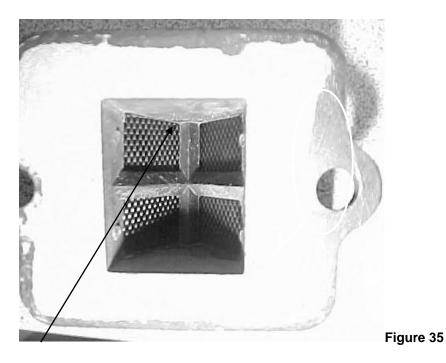
The presence of light indicates that the reeds should be replaced, or possibly turned over.
