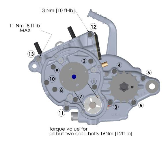
Torque the engine case bolts in the pattern shown above. The upper two bolts have a different toque value compared to the others.
