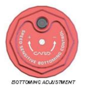
The Smart Leg cap is labeled "Speed Sensitive Bottoming Control", and this adjuster provides a range of control over how progressive the fork feels. Turning the screw clockwise increases the fork's resistance to bottoming, while turning the screw counter-clockwise decreases it. On the track, this effect will be felt on sections where the fork is forced to move very quickly such as on harsh landings or when traversing sharp edged bumps.
