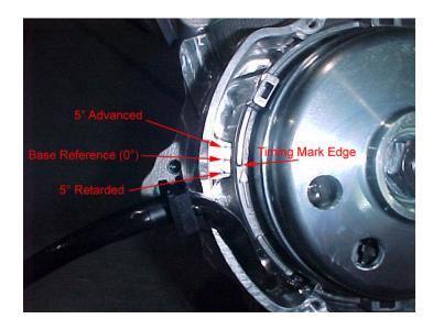
The center mark on the cases is the standard base reference timing mark  $(0^{\circ})$ , and the other two large marks are  $5^{\circ}$  advanced and retarded. The small timing marks between  $0 \& 5^{\circ}$  is  $2.5^{\circ}$ .
