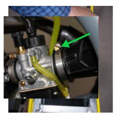
CAUTION: Pulling on the filter instead of pushing up on the boot may cause tearing of the filter.
