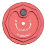
The speed at which the fork rebounds can be adjusted at the top of the conventional leg. Turning the adjustment screw clockwise slows the rate at which the fork extends after being compressed, and likewise, turning the screw counter-clockwise returns the leg to its extended position faster. As shown in the figure, 'S' (slower) and 'F' (faster) are etched into the cap as an adjustment guide.
