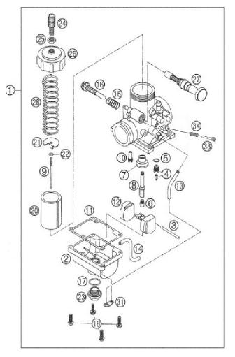
2. Raising the needle clip (this lowers the jet needle) one notch at a time on the slide.
