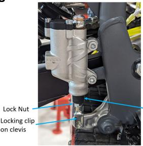
Threaded height adjustment shaft Under boot
