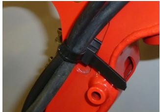
To disconnect these cable ties, use a screw driver as shown and push down on the short tab. The tab will be hidden from view by the cable tie strap.
