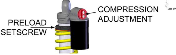
The Low Speed "L" adjustment is what controls how quickly the rear of the bike settles in the corners or how it settles in sweeping 'flat track' style corners whereas the High Speed "H" adjustment controls how the shock reacts to kickers. In "+" adds damping or slows it down, whereas out, "-" speeds up the shock or removes damping.
