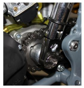
**NOTE:** The CFD hubs can be removed with the universal puller (MCMUTL70).
