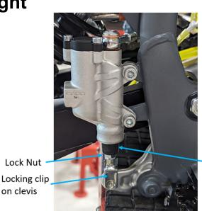
Threaded height adjustment shaft Under boot
