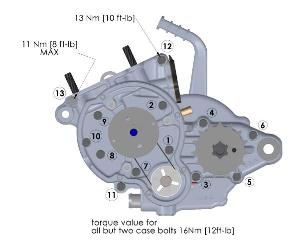
Torque the engine case bolts in the pattern shown above. The upper two bolts have a different toque value compared to the others.
