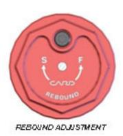
The speed at which the fork rebounds can be adjusted at the top of the conventional leg. Turning the adjustment screw clockwise slows the rate at which the fork extends after being compressed, and likewise, turning the screw counter-clockwise returns the leg to its extended position faster. As shown in
